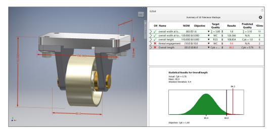
Oftentimes all the work creating these spreadsheets doesn't reveal the full story because a 1-dimensional stackup analysis may under-predict the actual assembly-level variation. EZtol helps you see the full story. The software warns if the tolerance stackup is not 1D in nature with a note that the results provided may underestimate the actual variation that will occur during production.
